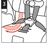
Reach under pad, pull one LATCH hook between rear harness slot and buckle strap.
